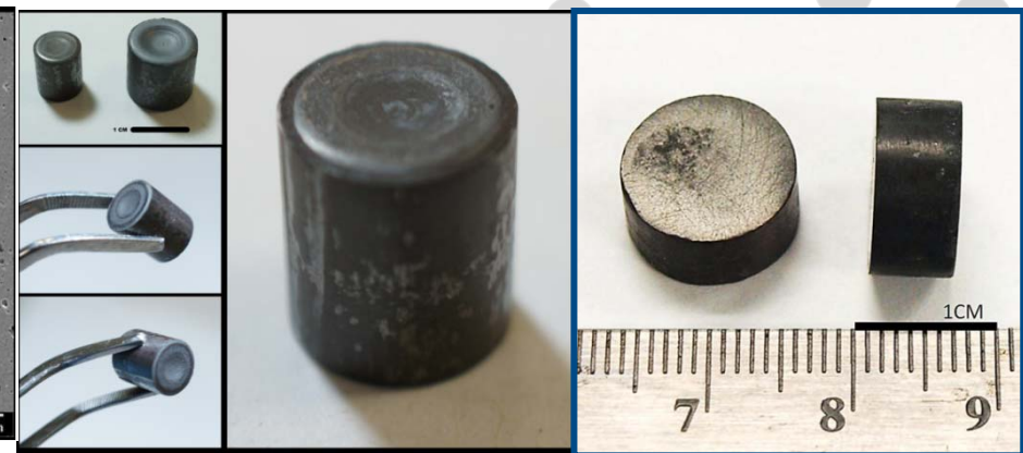
Figure 5: 17x17 \text{UO}_2 -SiC w pellets fabricated for irradiation in the ATR with a comparison of 15x15 and 17x17 sized pellets (top left)
