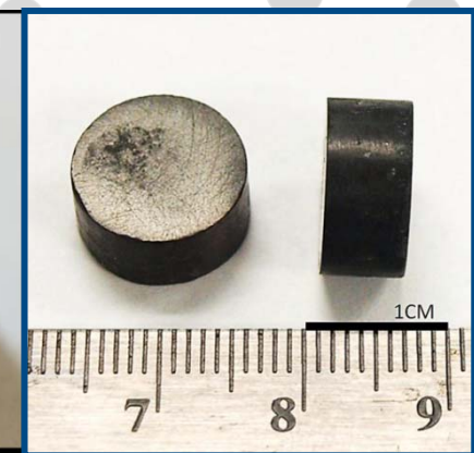
Figure 6: \text{UO}_2 – SiC research pellets utilized for various tests
